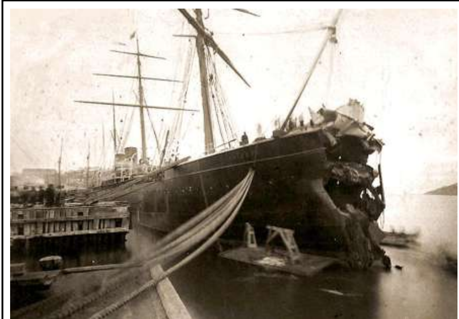
The S.S. Arizona in port, showing damage to her bow received when she struck an iceberg in the North Atlantic on the 7th of November 1879.
